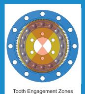
Characteristically, 30-40 percent of the teeth are engaged dependent upon the ratio, and load is shared amongst many teeth giving the drive its high torque capacity.
