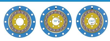
Example: with 100:1 ratio, 100 clockwise input motor rotations results in 1 counterclockwise output rotation.
