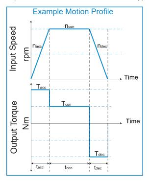
Review and note the following application data points for use in selecting the proper gearhead.
