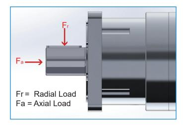
Radial and axial load maximums are listed under specifications by frame size. Radial load maximums are calculated with the load applied at key center. The average radial and axial forces can be calculated using the equations provided below. If the forces calculated exceed maximums for the gearhead, select a larger size or contact Conic Systems for further assistance.
